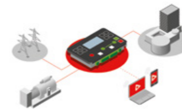
IT Controllo remoto via ethernet, rete 4G e controllo posizione GPS EN Remote control via ethernet, 4G network and GPS position control FR Commande à distance via Ethernet, connexion 4G, et contrôle de position GPS
